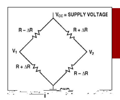
$$V_1 = \frac{\overline{R_3}}{R_2 + R_3} V = \frac{1}{2} (1 + \frac{\Delta R}{R}) V$$
